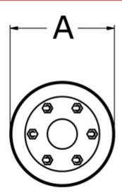
A = 157 D1 = 55 D2 = 55 L = 170 Nom. torque NM (Tkn) = 800
